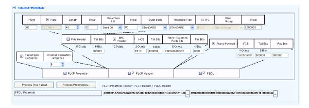
For a packet, you can set the <u>PLCP Preamble (see page 85)</u>, <u>PLCP Header (see page 86)</u> and <u>PSDU (see page 87)</u> parameters. Many parameters have either a dropdown list to select values from, or a text box to enter values (in hexadecimal or binary). Other parameters open the next level of choices or a dialog box.
