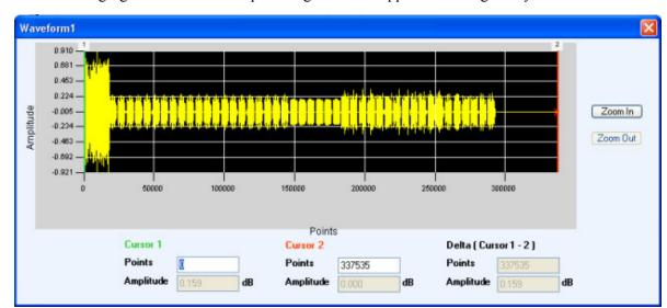
The following figure shows an example of a gated noise applied to a range of symbols.
