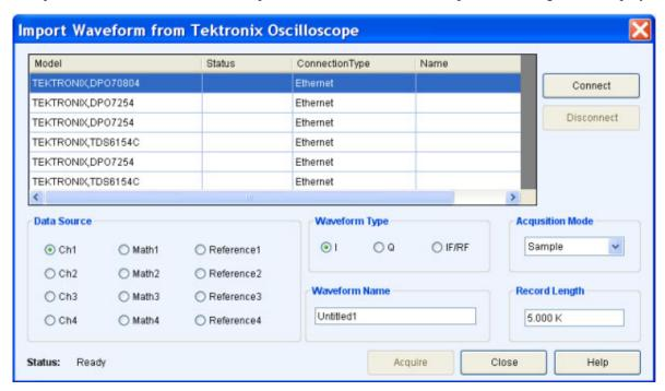
A table displays a list of oscilloscopes on the network. Select an oscilloscope in the table and click Connect to connect to it. You can connect to more than one oscilloscope at a time. Click Disconnect to disconnect from an oscilloscope.
