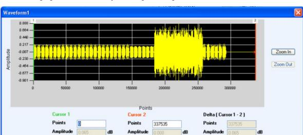
The following figure shows an example of a signal with gated noise.
