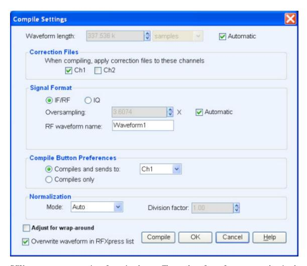
RFXpress supports generation of two signal types. The number of waveforms generated varies depending on the signal format selected.
