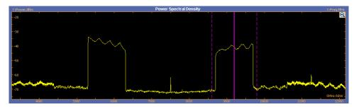
RFXpress can create a signal above Nyquist (Fs/2) using undersampling. Calibration would allow you to get a flat frequency and linear phase response in the first image of the signal, in this example at 9.2 GHz. RFXpress also provides for swapping of I and Q (in the IQ impairments tab) and phase inversion of I and Q (in the Compile Settings dialog box) to create undersampled signals.
