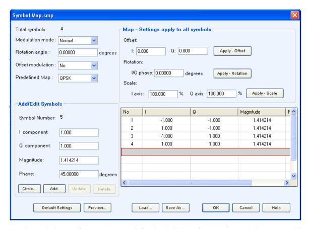
Use the symbol map editor to create user defined modulation schemes. The Symbol Map created is stored in a binary format. This is useful for unsupported modulation schemes and to introduce impairments with the simulated waveform.
