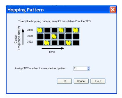
To customize a hopping pattern, set the TF Code to User Defined. You can define a hopping pattern by clicking the black squares in each column. This sets the frequency at which a packet is transmitted for each band in a band group. After you have defined the hopping pattern, assign a TFC number (between 1 to 15) to the pattern and click OK.
