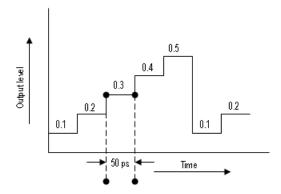
In the interleave mode, alternate samples are output from each channel. The samples are distributed between the two channels as shown below:
