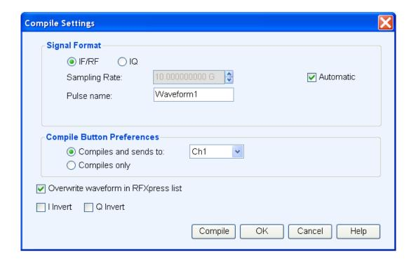
RFXpress supports generation of two signal types. The number of waveforms generated varies depending on the signal format selected.
