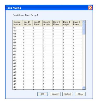
The amplitude values are relative to the amplitudes specified for each band. The tone nulling value ranges between -40 dB and +20 dB. For example, if a carrier or tone value is set to -40 dB, the amplitude of the tone is 40 dB less than that specified for the band to which it belongs. The phase value ranges from -180 degrees to +180 degrees.
